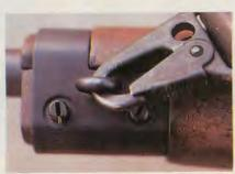
ABOVE: SL7 front barrel band with retaining pins and front sling swivel.
